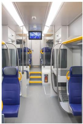
vestibules are ideal for the shorter journeys, typical of suburban traffic. The seats are equipped with power sockets for PCs, tablets and cell phones. The lighting is optimised by the large windows that let in more natural light, and passenger circulation is facilitated by wide corridors that are also suitable for people with reduced mobility.
